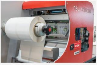
• Feeder up to 300mm rolls & Web cleaner to guarantee consistent results.
