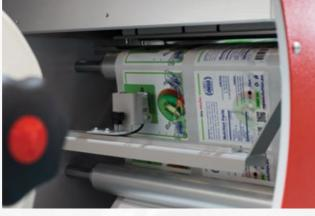
• Light sensor for reading pre-diecuted label rolls.
