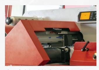
· Camera for single mark detection enables faster cutting process.
