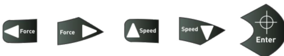
In order to set the correct starting point for plotting, in offline mode, move the cutter head and foil in such a way, that the laser point is located in the so-called start box in front of the bar code on the inserted medium. Now confirm the zero point by pressing the crosshair, which will cause the device to automatically switch to online mode.
